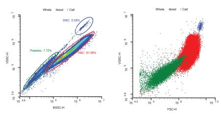
Dual SSC with V-SSC and B-SSC are used to separate whole blood into platelets, red blood cells, and white blood cells without the need for any lysis protocols. Note: Optimization may be required.
