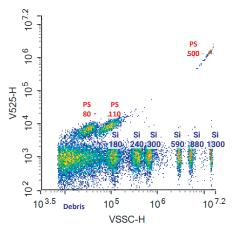
ApogeeMix beads, a mixture of polystyrene fluorescent and silica beads, were analyzed using V-SSC and fluorescence. NIST Traceable Particle Size Standards were analyzed using either V-SSC for smaller particles and B-SSC for larger particles.
