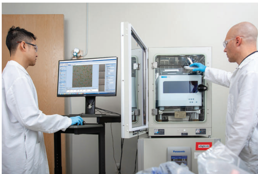
Figure 5. An Agilent xCELLigence RTCA eSight instrument and its control unit are housed inside and outside an incubator, respectively.
