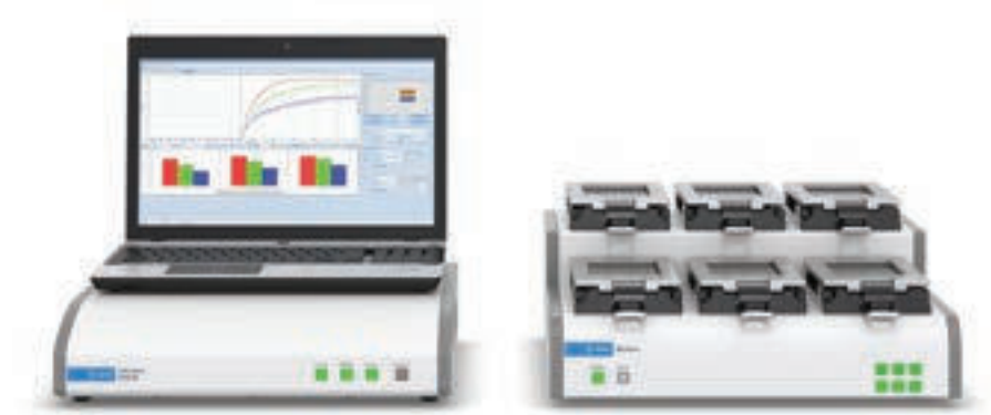
Figure 2. Example of an Agilent xCELLigence instrument. xCELLigence instruments are available in different formats (16-, 48-, 96-, and 576-wells). The instrument shown contains six cradles, each of which houses an electronic 96-well microplate. The plate-housing portion of the instrument is placed inside a standard tissue culture incubator, while the analyzer and control unit (a laptop computer) are housed outside the incubator. All six plates can be monitored simultaneously and independently of one another, maximizing throughput and flexibility.
